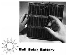
solar cells are  $6 \ cm \times 1.4 \ cm$  and the spacing between them 0.33  $\ cm$ . The efficiency is  $\eta = 6\%$
